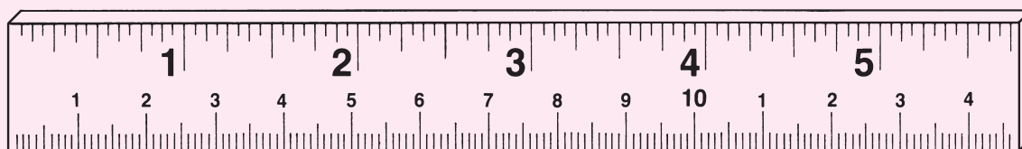
Portion of metric ruler, with inches (upper scale) and centimeters (lower scale)
